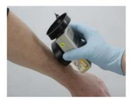
Perform a detailed scan for external contamination. Scan body slowly at distance of 1cm (approx 3 mins)
